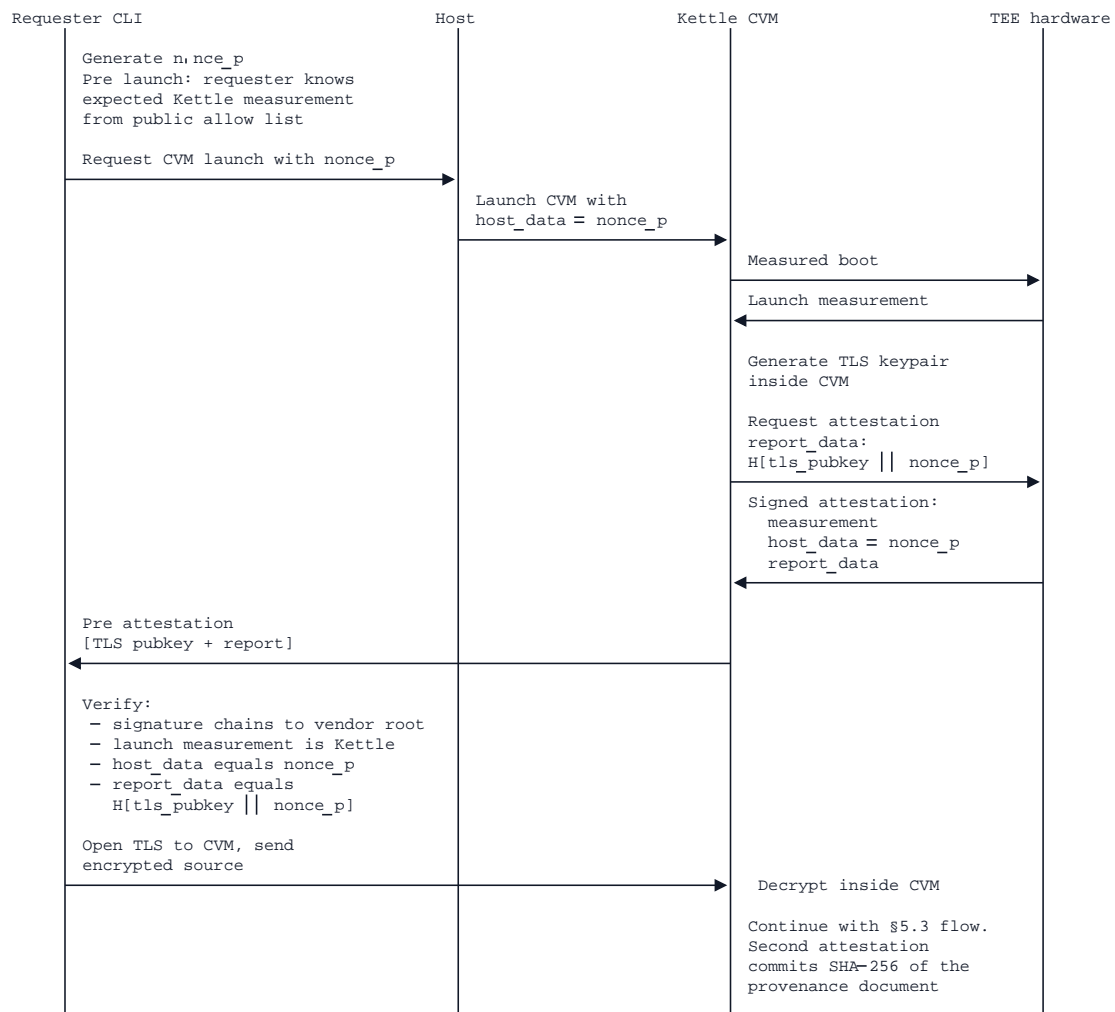
Figure 10. Pre-attested confidential build. The requester generates a single nonce that the hypervisor commits into the CVM’s host_data field at launch and that Kettle inside the CVM also includes in report_data . The first attestation therefore proves three things at once. The CVM is running Kettle code, it was uniquely launched for this requester, and the report itself is fresh. Source is then delivered over a TLS channel terminated inside the CVM, and the standard §5.3 attestation over the provenance document follows.
